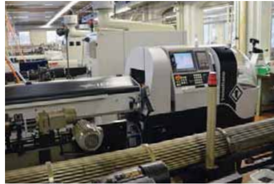
The SwissNano machine and lemca bar feeder have a very small footprint. The director plans to set up machines equipped with 2 m bar feeders to increase the number of machines installed.
