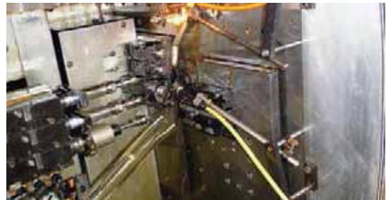
Deco 10 sawing a connector contact.
