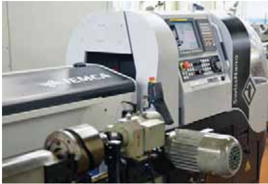
The SwissNano machine and lemca bar feeder have a very small footprint. The director plans to set up machines equipped with 2 m bar feeders to increase the number of machines installed.
