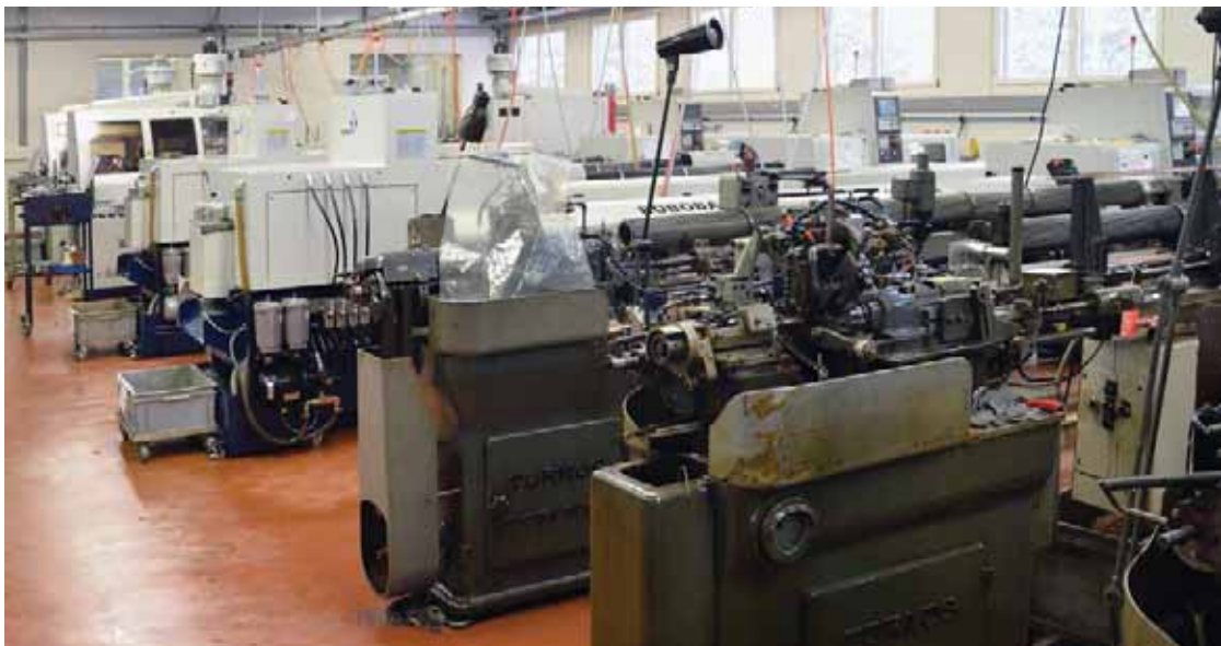
The Ultra workshop has a range of different machines, which means that the best machine can be chosen for the part to be made. For lead times of less than a week, the SwissNano has replaced the existing cam-type machines.
