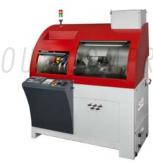
**The escomatic EC 08** is the logic and innovative evolution of the well proven D6 series with CNC technology. The automatic turning centre manufactures cost effective small as well as large batch sizes with diameters up to 8.0mm. Equipped with a tool head with four cutting tools, two capable of working simultaneously, and up to 12 tooling positions for secondary operations, the turning-centre works with commercially available inserts as well as Esco special cutting tools.
