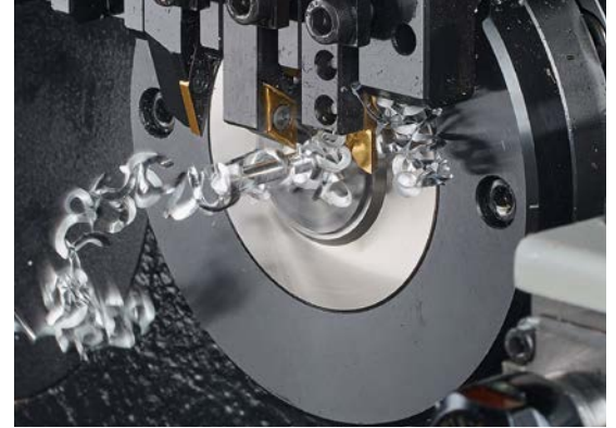
Without active chip breaker
