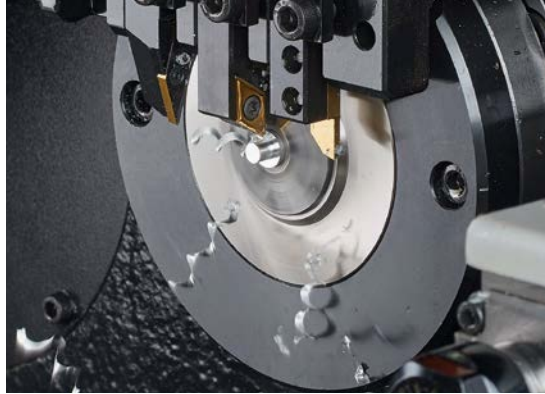
With active chip breaker
