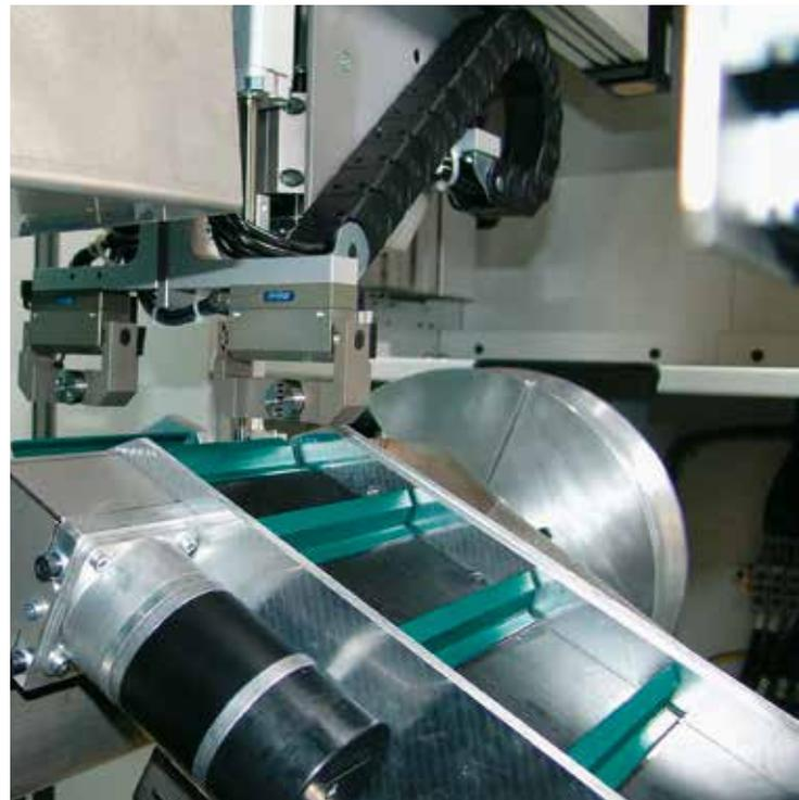
Precision and the visual appearance of the parts being manufactured in today's market are becoming more and more stringent. Dents, marks and flaws are no longer permitted. In order to meet these requirements, Tornos developed a dual parts handling system, which picks up the parts and conveys them directly to the machining area and then conveys them outside of the machining area.
