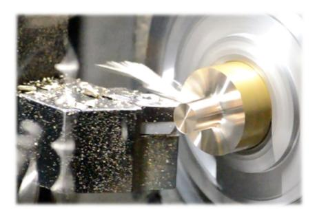
2) "TWISTER" turning with a single tool in finishing mode with a very small and very long diameter
