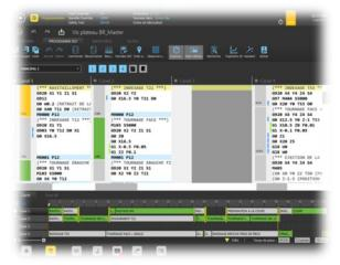
2) A machine manipulation interface which replaces the FANUC pages called "TISIS Pilot".
