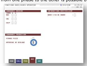
This principle allows you to position your tools extremely close to the rapid-feed material, without risking contact thanks to a more distant approach when you are adjusting your tools.
