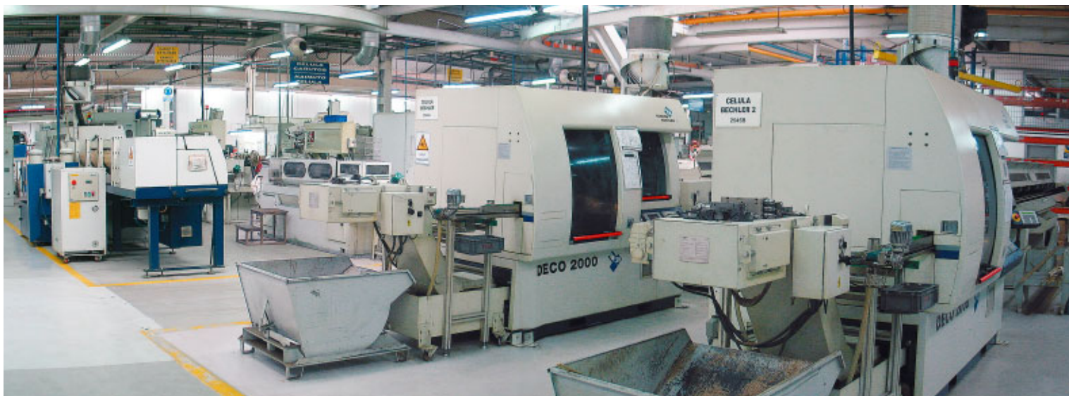
The «Bechler unit» consisting of two DECO 20a machines.
