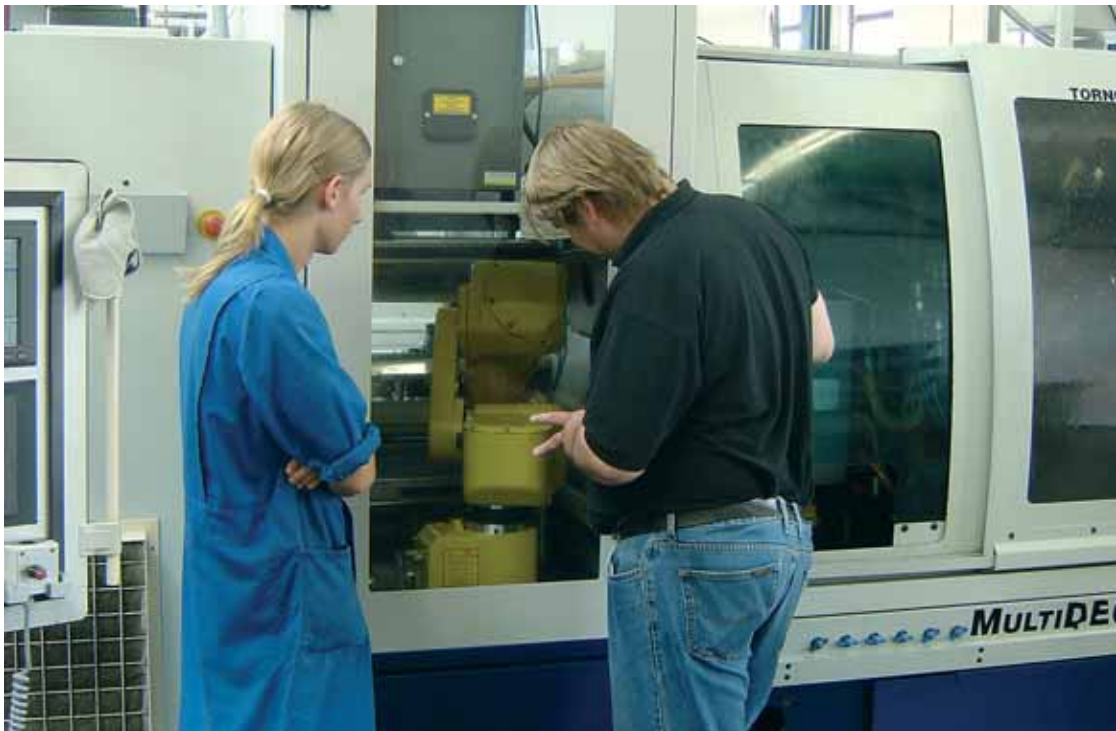
Tornos CNC multi-spindle automatic turning machine with integrated robot cell manufactured by Handling Tech.
