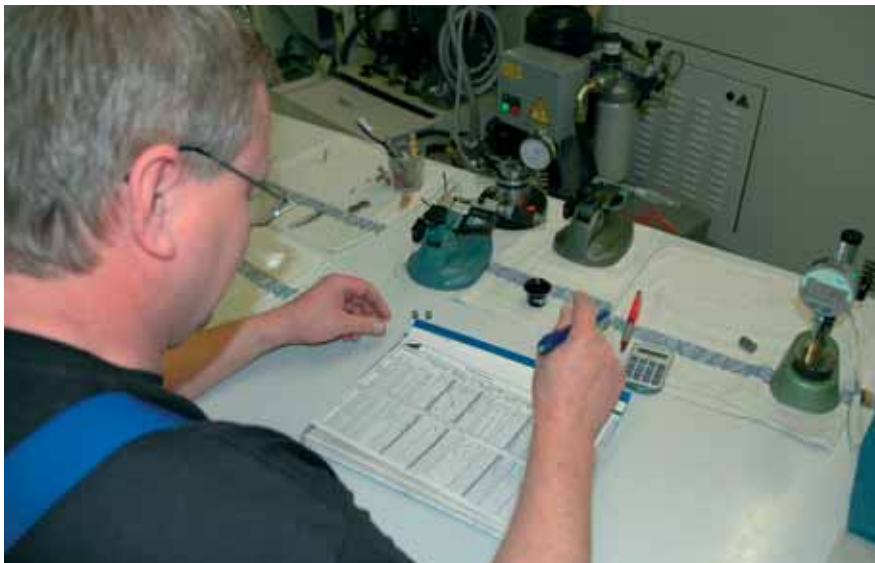
Precision to the nearest hundredth is now seldom sufficient. Through a process of regular measuring checks with all results recorded in a definitive measuring log during volume production, the machine operator always knows exactly how things stand at any point in time.
