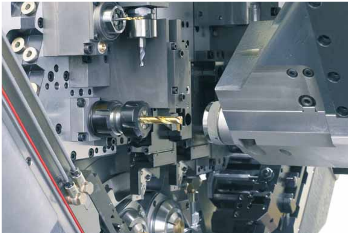
With 5 counter-operation tools, MultiAlpha can also perform complex counter-operations.
