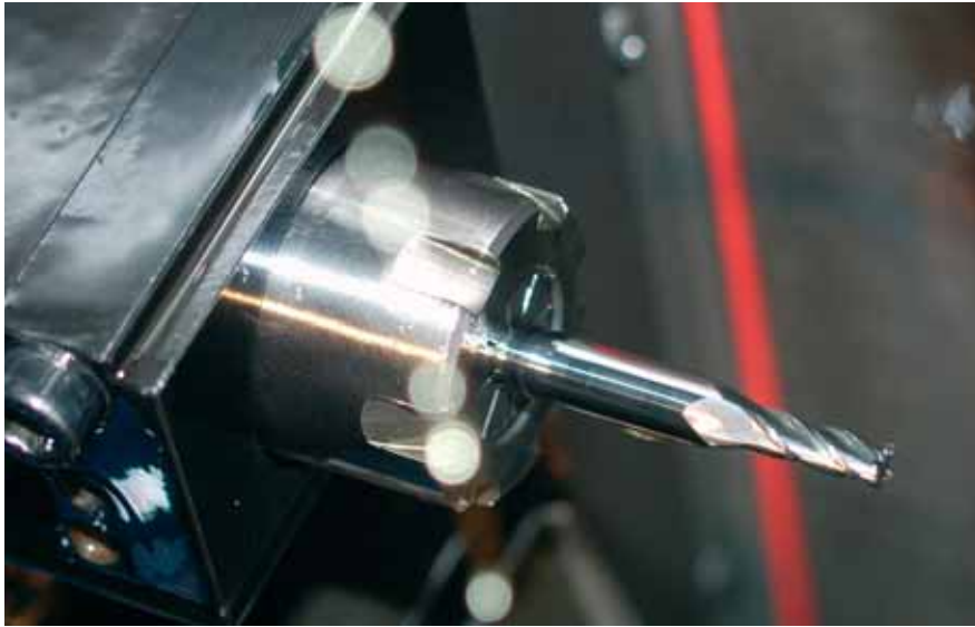
The solid hard metal milling tool rotates at approximately 6000 rpm and removes material for the tapered external hexagon in a single pass on the medical technology machine tool.
