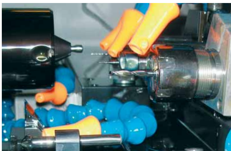
Counter-operation machining of Torx.
