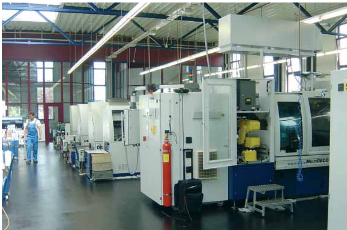
In the clean and generously proportioned factory building, Tornos CNC multi-spindle and CNC single-spindle units stand in series and operate reliably round the clock.
