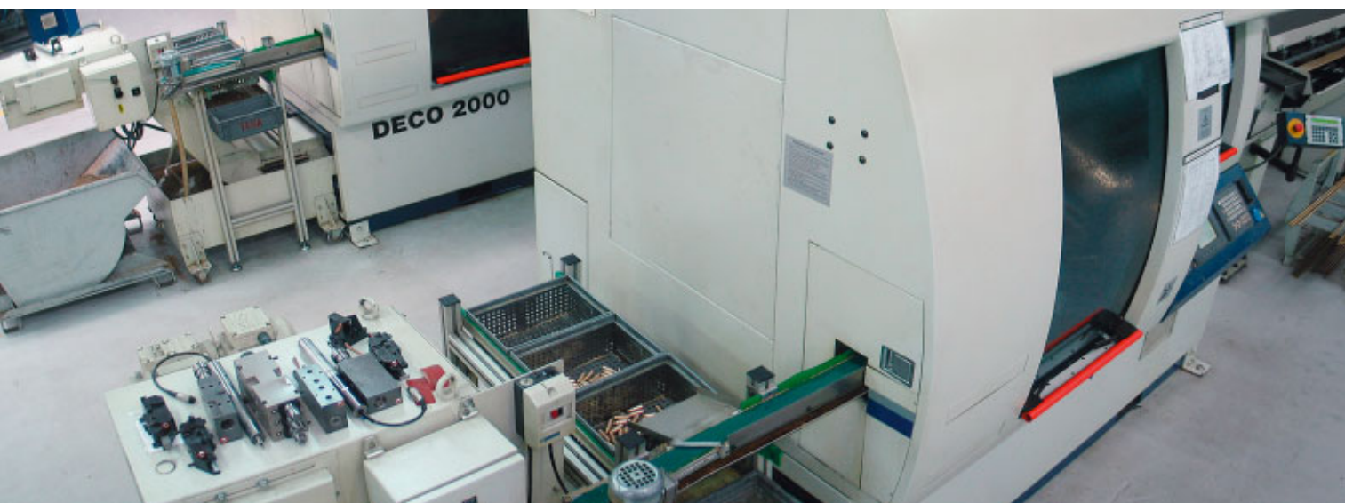
DECO production unit. The equipment and tools ready to be fitted for machining the next series can be seen in the foreground.
