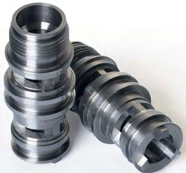
AISI 1215 carbon steel industrial hydraulics components machined on the Tornos DECO 20
