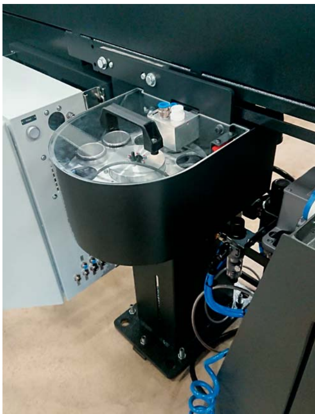
A vacuum carousel specially developed by Tornos for the reliable recovery of ultrasmall parts thanks to a controlled suction system
