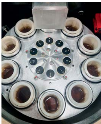
A vacuum carousel specially developed by Tornos for the reliable recovery of ultrasmall parts thanks to a controlled suction system
