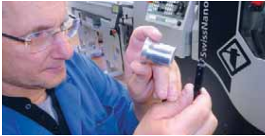
The way in which a tool wears out and the colours it presents can provide bar turners with a lot of important information.
