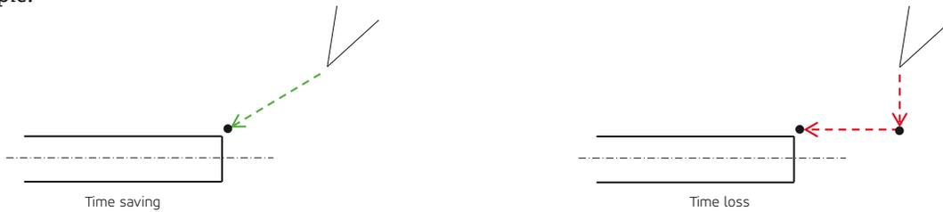
It is also possible to approach the tool simultaneously in the linear and rotary axes (e.g. Y, Z + C).
