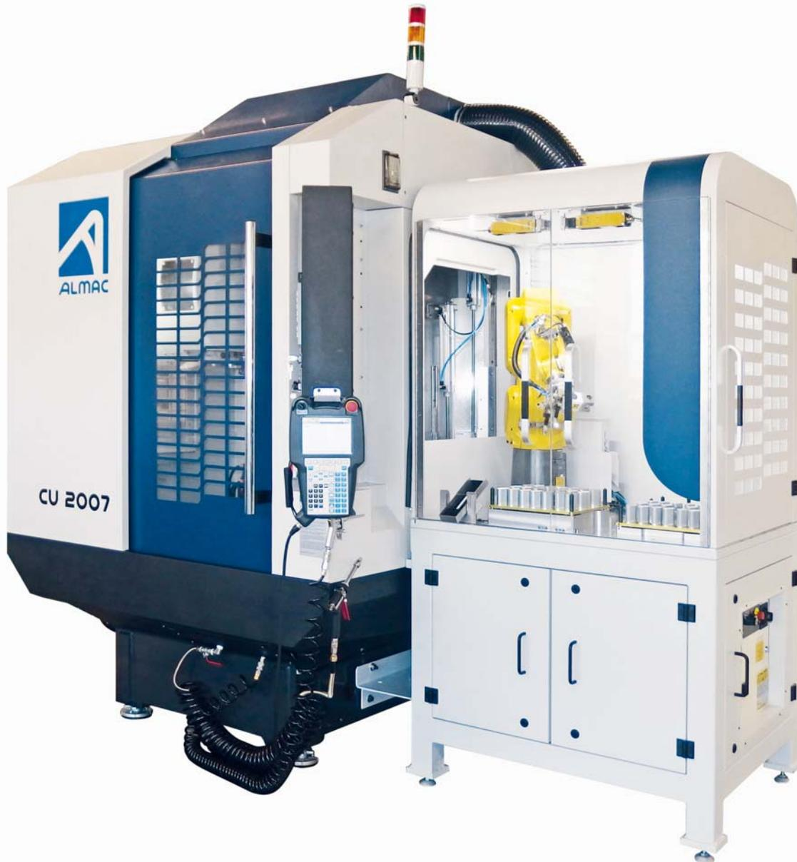
located at the heart of the machining area. Once the first part has been finished, the manipulator arm picks it up while the magazine opens. The workpiece is deposited in an empty position and the arm picks up the workpiece to be machined next and loads it onto the fixture. The workpiece is clamped and the magazine closes. The workpieces in the magazine are well protected and minimum loading and unloading times are achieved.
