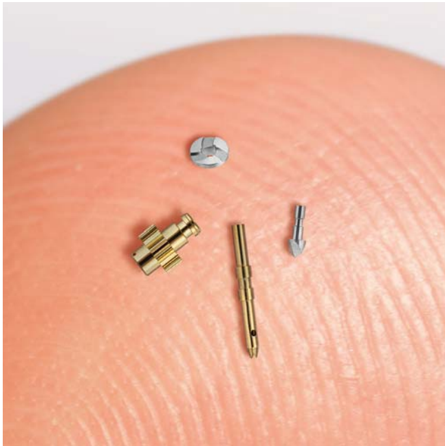
The parts produced through micro-turning may not be very complex in terms of geometry. However, their production with the required quality and precision and at the agreed price while heeding a specific deadline is a real day-to-day challenge.
