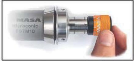
Precise adjustment of the clamping force with the Micrograd™ Dial Wrench
