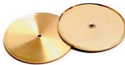
This machined test piece for the comparison of materials reflects typical watchmaking problems.
