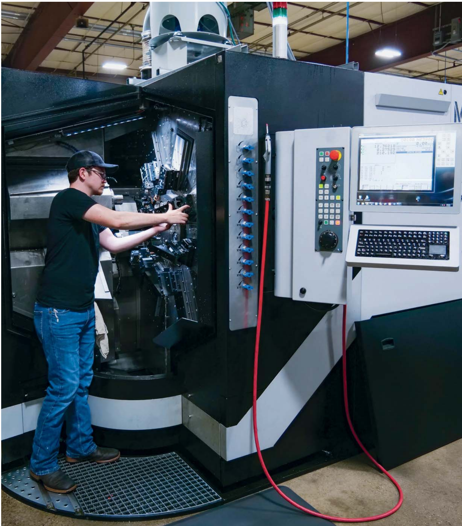
As a job shop, Mitotec Precision continues to identify ways to speed changeovers for jobs that run across its two CNC multispindle machines for operators such as apprentice-now-employee Trevor Hutchins. Batch sizes of 20,000 parts is its sweet spot for these machines. (Photo Credit: Mitotec Precision)
