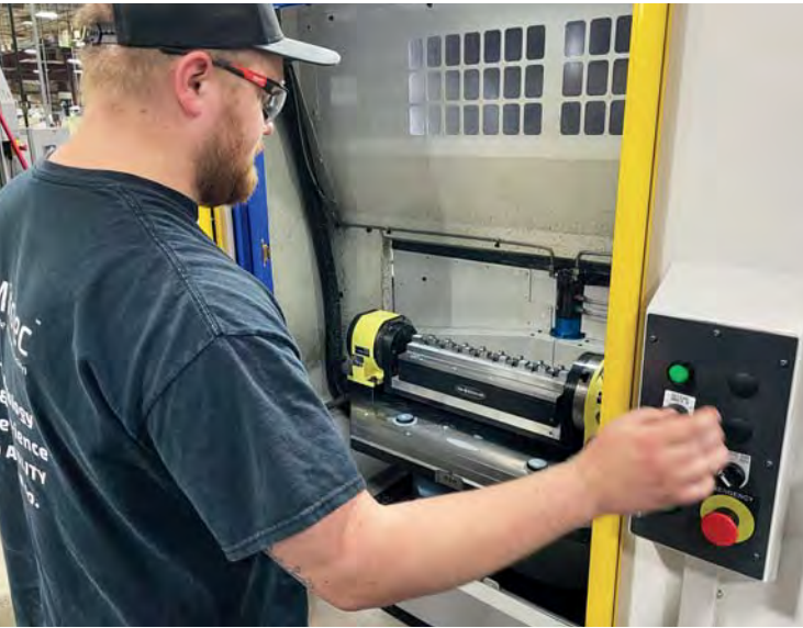
The CNC multispindle's opened-up additional capacity on Mitotec Precision's four VMCs that were previously used for second-op work. Now, the shop is using machines such as this Brother VMC with pallet changer and hydraulic workholding for production work.
