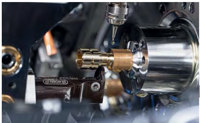
The S224 prism-guided precision insert is used for threading.
