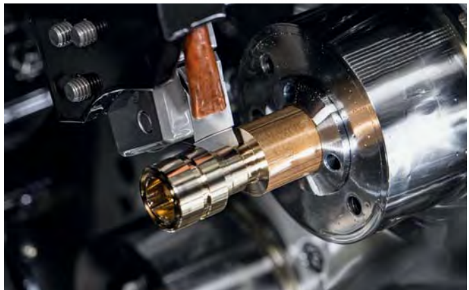
The form groove is made with the 315 System, which is characterized by high changeover accuracy.
