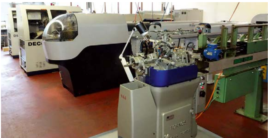
The workshop of Gérald Badan SA comprises machines of three generations that enable the company to meet any demands up to diameters of 10 mm.
