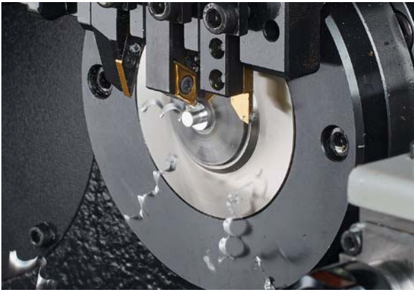
With active chip breaker
