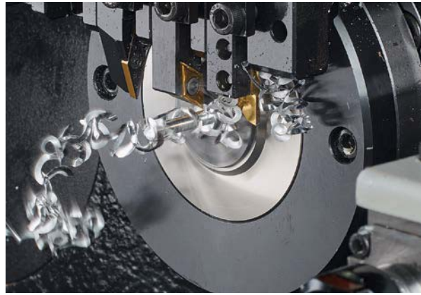
Without active chip breaker
