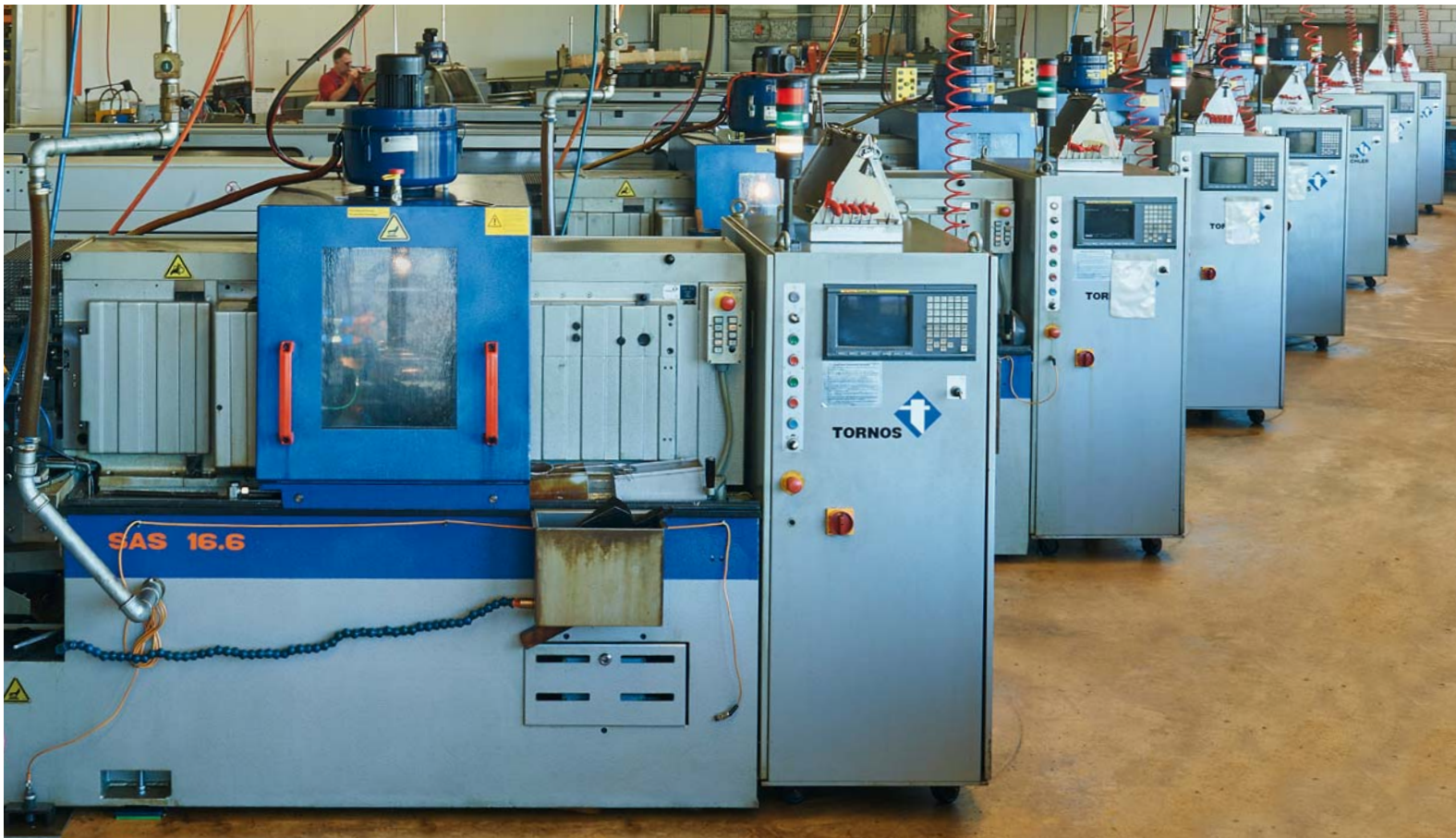
A total of 17 cam-controlled multi-spindle automatic lathes SAS 16.6 and AS 14 by Tornos are used at RB-Cema.
