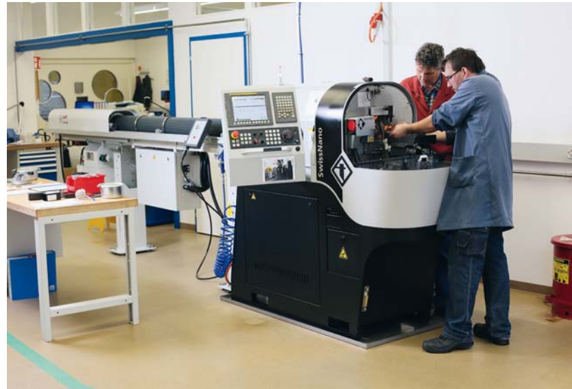
Teacher and apprentices: the SwissNano machine on which the apprentices are especially taught in gear hobbing.
