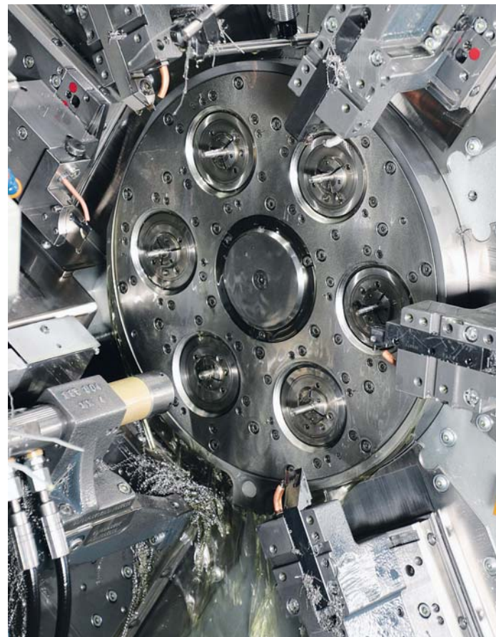
The work envelope of the MultiSwiss with automotive components in each spindle.
