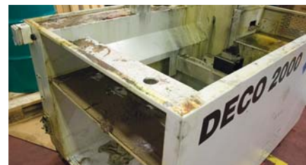
In case of a complete overhaul, the machine is fully disassembled and reconditioned.
