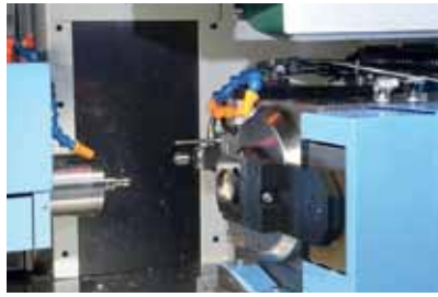
The counter spindle waits for a plate to machine it on face two...
