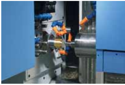
View of the main spindle: the machine is ready to machine face one of a new plate directly on the bar.
