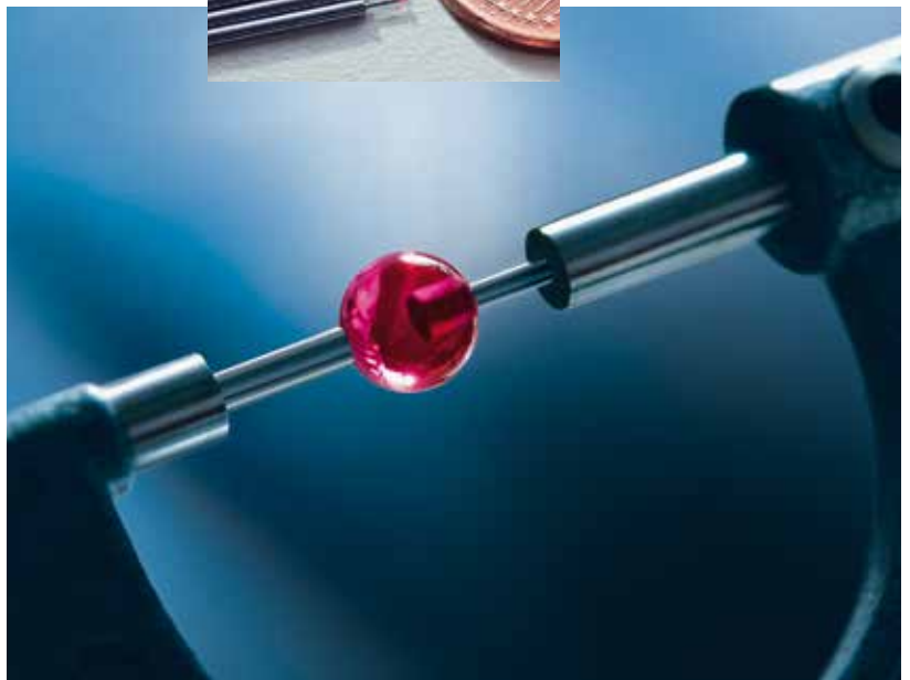
This probe ball made from ruby has an extremely high circularity (grade 5), which corresponds to 0.08 to 0.13 µ. Drilling blind holes for mounting the probe ball is one of itp's specialities and requires a great deal of knowledge and skill.
