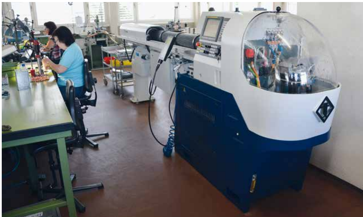
For testing purposes, the SwissNano machine was installed away from the bar turning workshop. Its compact size and its design mean it will fit in any workshop. As there is no rear access, it can even be installed against a wall.
