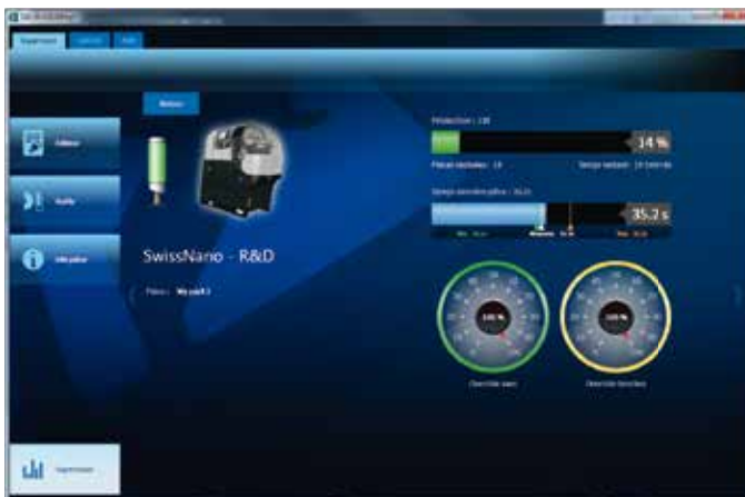
Detailed monitoring of a machine in real time and monitoring of the production status. The drawing for the current workpiece can, for example, also be displayed.
