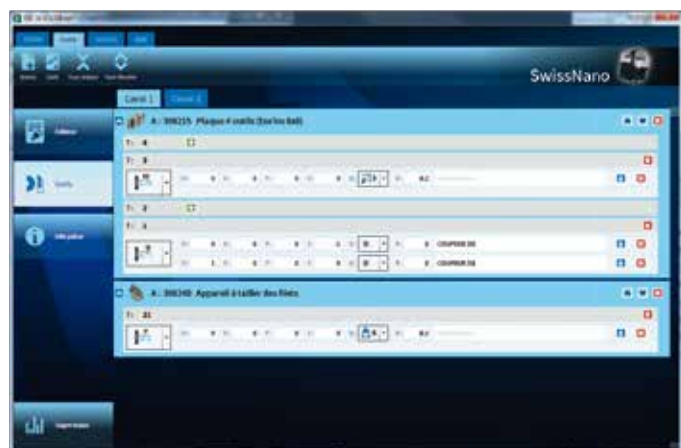
ISIS proposes default tool geometries; the user is free to correct them if necessary.
