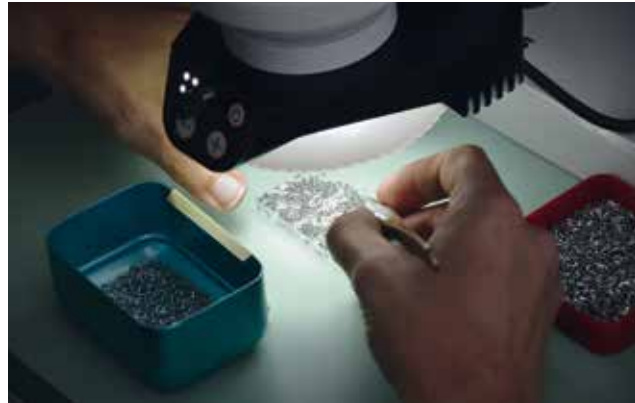
In order to offer its customers a complete solution, the company includes various departments in addition to bar turning, for example, polishing or rolling. The barrel arbors produced on the SwissNano are tempered (by a partner company), then rolled and checked on site.
