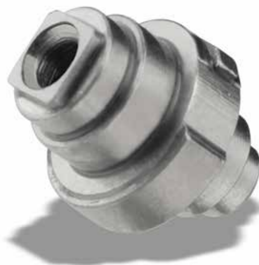
The barrel arbor is a part at the limit of the SwissNano's complexity. To increase the range of operations available on the SwissNano, Krattiger will soon be testing the cutting device.
