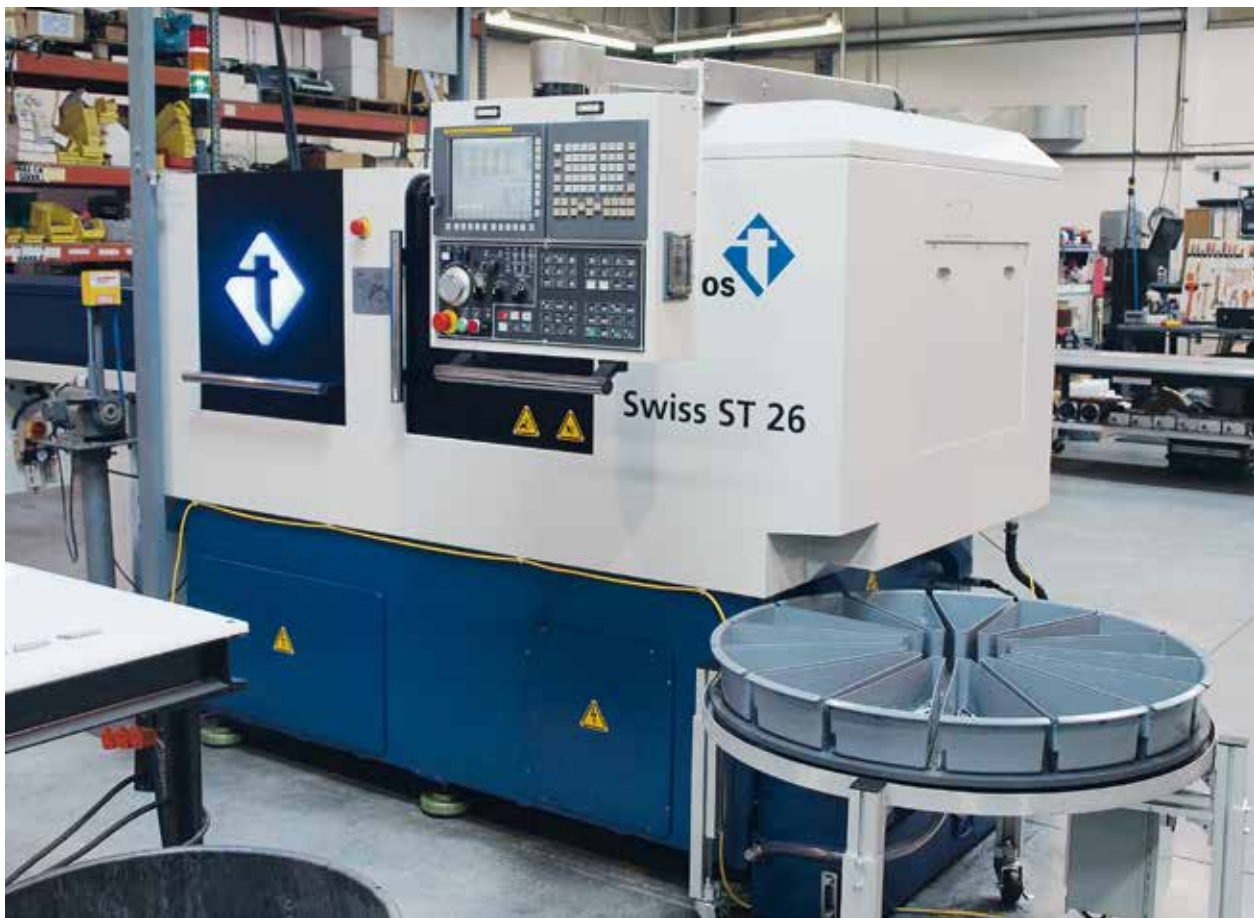
Swiss ST 26 with parts carousel shown.
