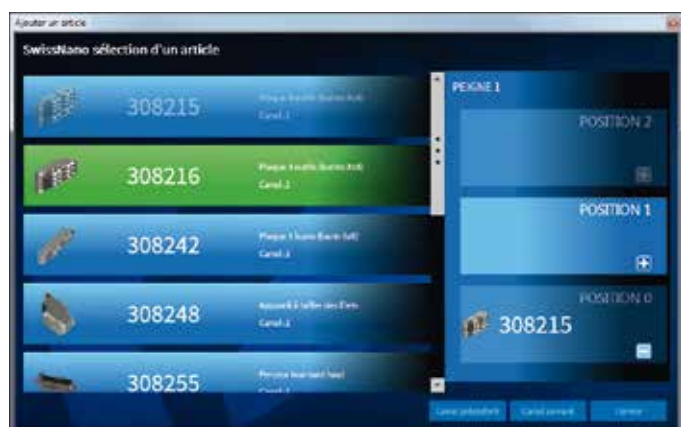
Selection of a tool on the SwissNano; unavailable tools are greyed out. Mounted tools are shown in dark blue, and users have given this solution a unanimous thumbs up!
