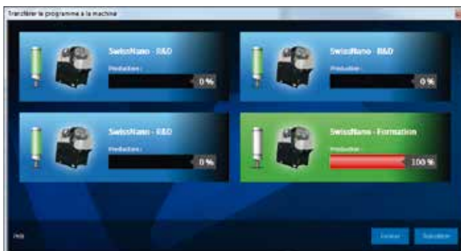
Virtual program transfer. The program can also be edited on the machine and transferred intuitively back to the computer.
