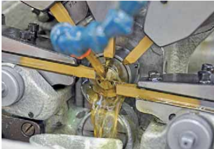
The choice of machining fluid impacts directly on tool productivity and lifetime.
