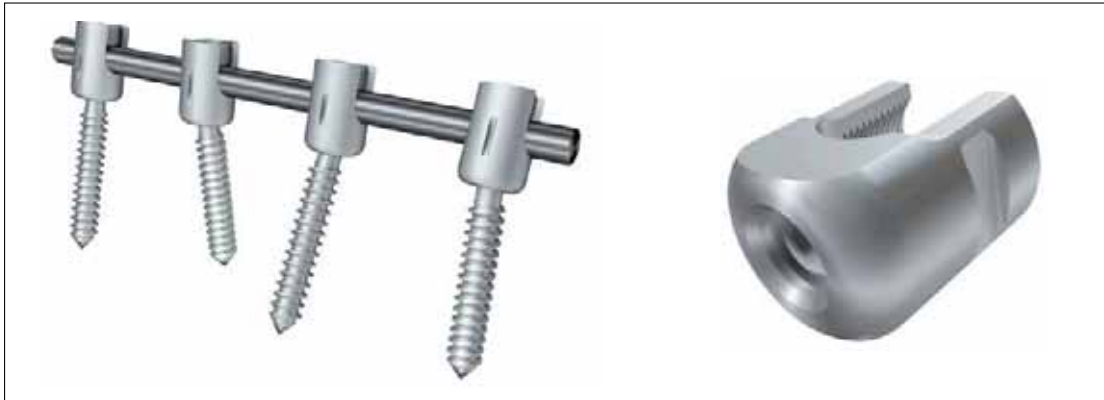
Tulip heads for spinal parts are ideal for machining in a modern sliding-head machine. Milling is a dominant machining method to arrive at the head configuration and one that needs careful optimization. The combination of the right solid-carbide endmill and tool-path are decisive as regards efficiency and security. As important is the optimization of turning, thread-turning and grooving with the right tools. The resources of a modern sliding-head machine can be put to very advantageous use, resulting in good manufacturing economics.
