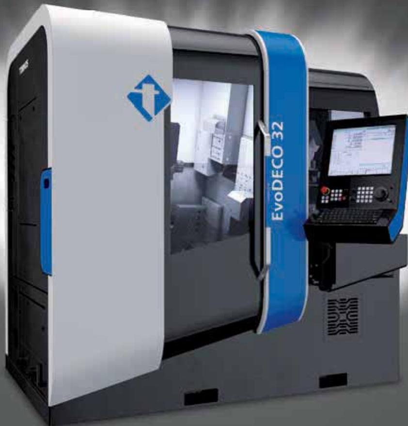
Featuring a full range of basic equipment, the new EvoDECO 20 and EvoDECO 32 guarantee optimal productivity thanks to their unique kinematics. Equipped with a reinforced structure, they also offer the most powerful spindles on the market (9.5/12.8 kW). With identical power for both primary and secondary operations, they deliver constant torque regardless of the rotation speed. For more information on the EvoDECO 20 and EvoDECO 32, visit [www.tornos.com](http://www.tornos.com)
