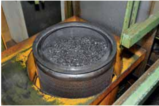
The Motorex Ortho NF-X cutting oil is especially low in volatility and can be easily centrifuged from the swarf. In this way, oil discharge can be reduced to a minimum and fresh oil is only added from time to time.
