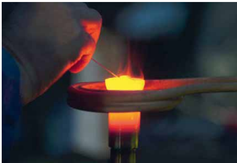
Welding of tungsten carbide in the guide bush.
