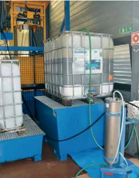
The reclaimed cutting oil is cleaned using a filtering system and fed into the machine tools together with a proportion of fresh oil.
