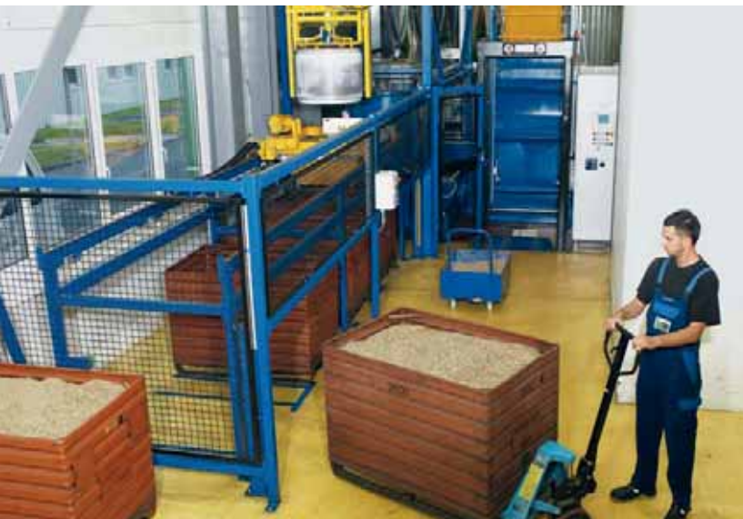
The switch to a single cutting oil also made it easier to reclaim oil using the fully automatic chip centrifuge.
