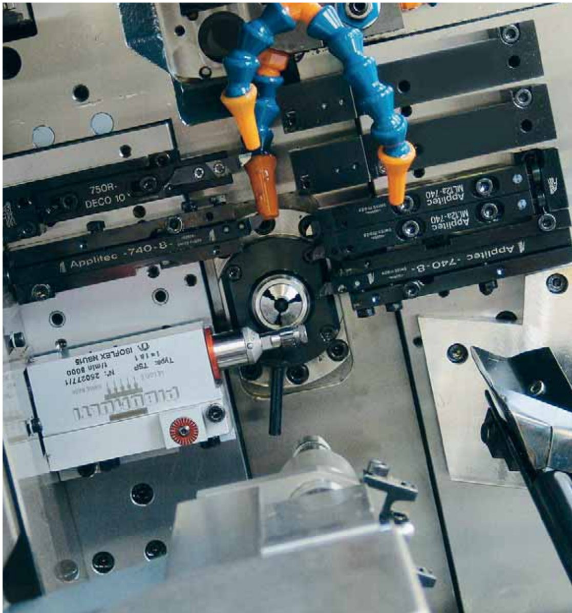
The kinematics of the machine are based on the success behind the Deco 10, namely four independent and simultaneous tool systems.
