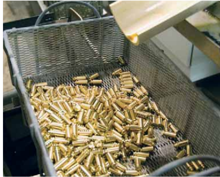
One of WB's Tornos CNC multi-spindle's two gantry pick-off spindles is visible at right. The discharge chute (left) carries two finished parts per drum index using the machine's 2 × 4 machining capability
