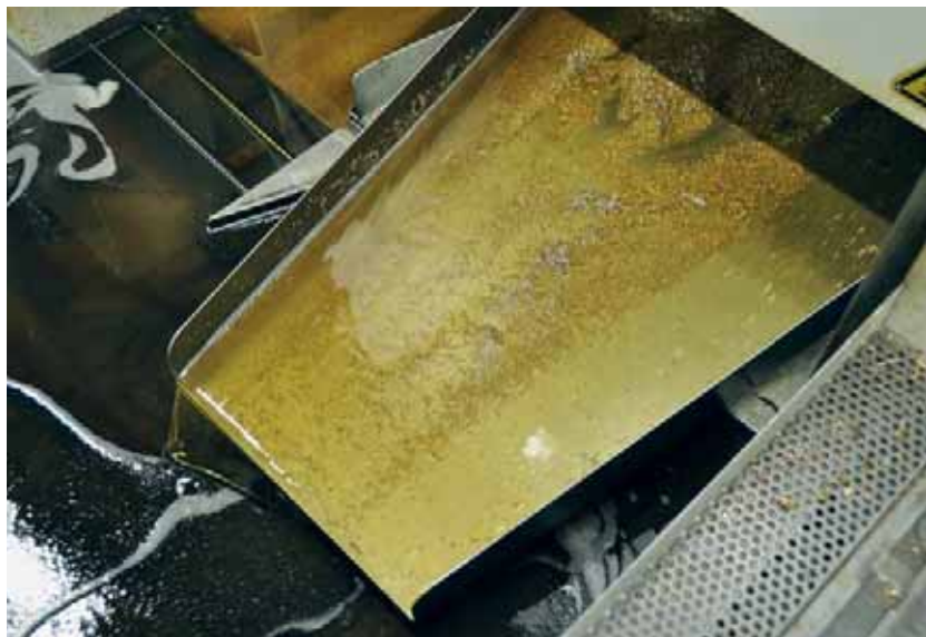
Chips are produced by the ton during the manufacturing process at BEC. The recycling thereof and the reclamation of the cutting oil that is used are decisive for the calculation.
