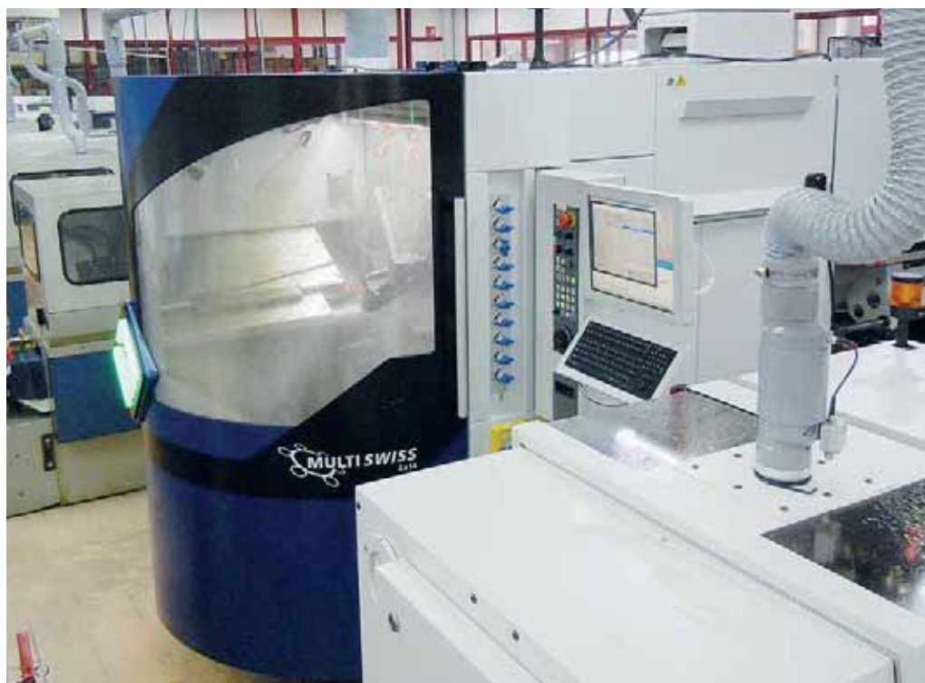
In terms of space requirements, the MultiSwiss is a straight replacement for an ENC single-spindle lathe.
