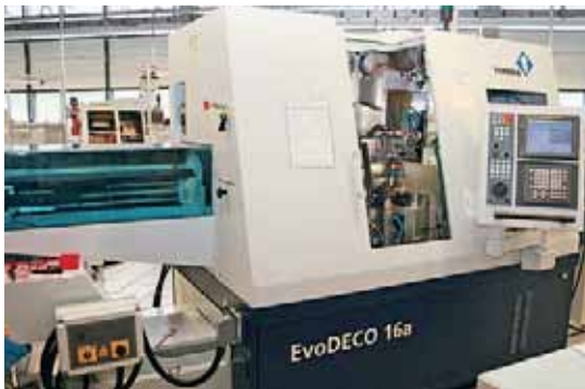
The clearly visible recess above the working area is attributable to the integration of this part of the casing in the sliding doors. A feature that is greatly appreciated by the turning machine operators.
