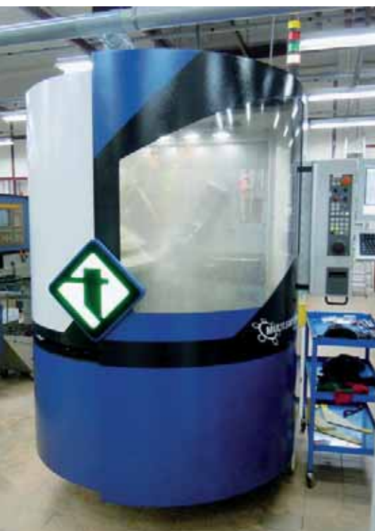
In terms of space requirements, the MultiSwiss is a straight replacement for an ENC single-spindle lathe.
