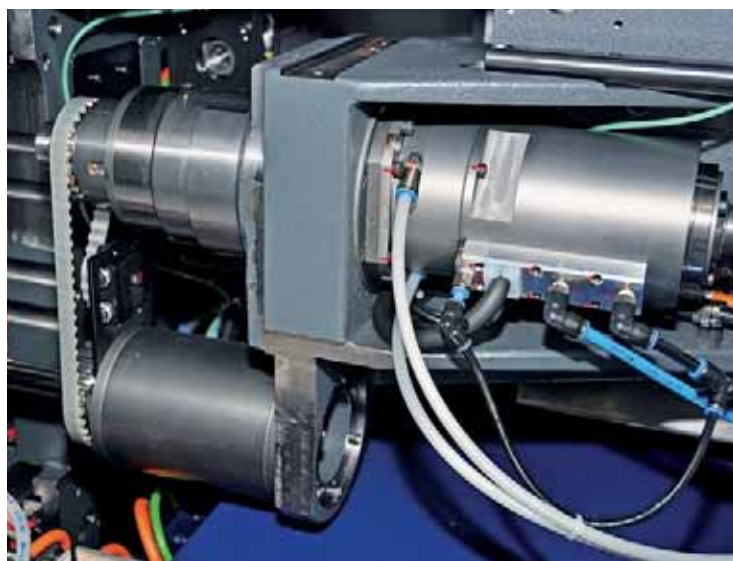
Designed for high performance, the synchronous motorised spindle is an important factor for success. Good to see: the two transparent supply lines for the spindle cooling fluid.
