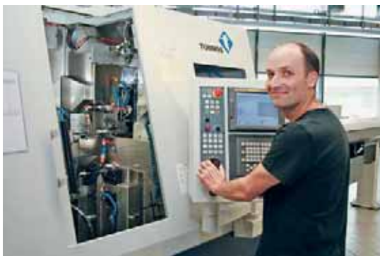
Eric Pesselier welcomes the extra ease with which the automatic turning machine can be set up now that the control is built onto a rotary arm.
