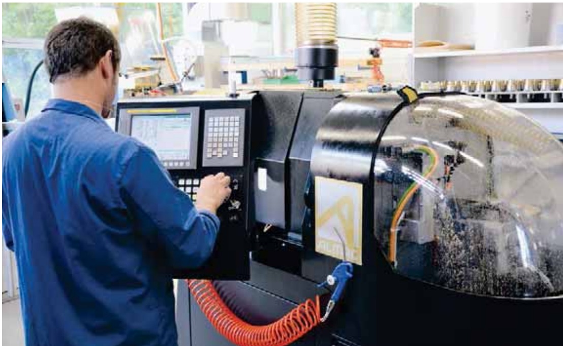
The BA 1008 is connected to Metalem's centralised oil mist suction system.
