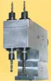
Polyvalent drilling and milling head for heavy machining with speed-reducer Usable with or without over-arm
