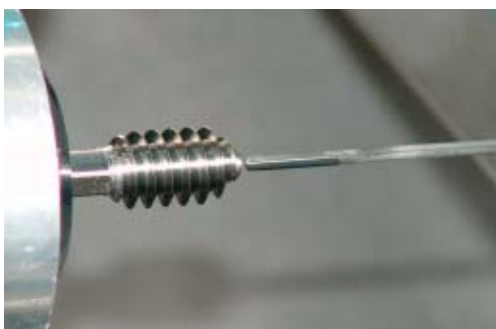
Back-operation high pressure drilling at 120 bar using the guide bush.
