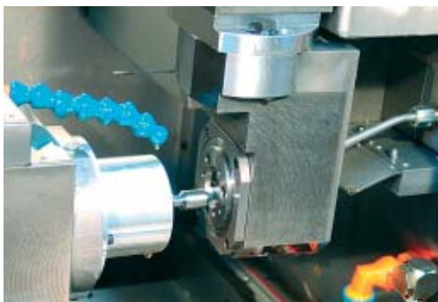
Back operation thread whirling (3 rough working passes and 1 finishing pass) in hidden time.
