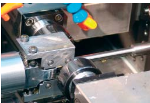
External hexagon milling with 2 tools simultaneously and end piece support.
