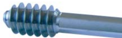
Back operation thread whirling (3 rough working passes and 1 finishing pass) in hidden time.
