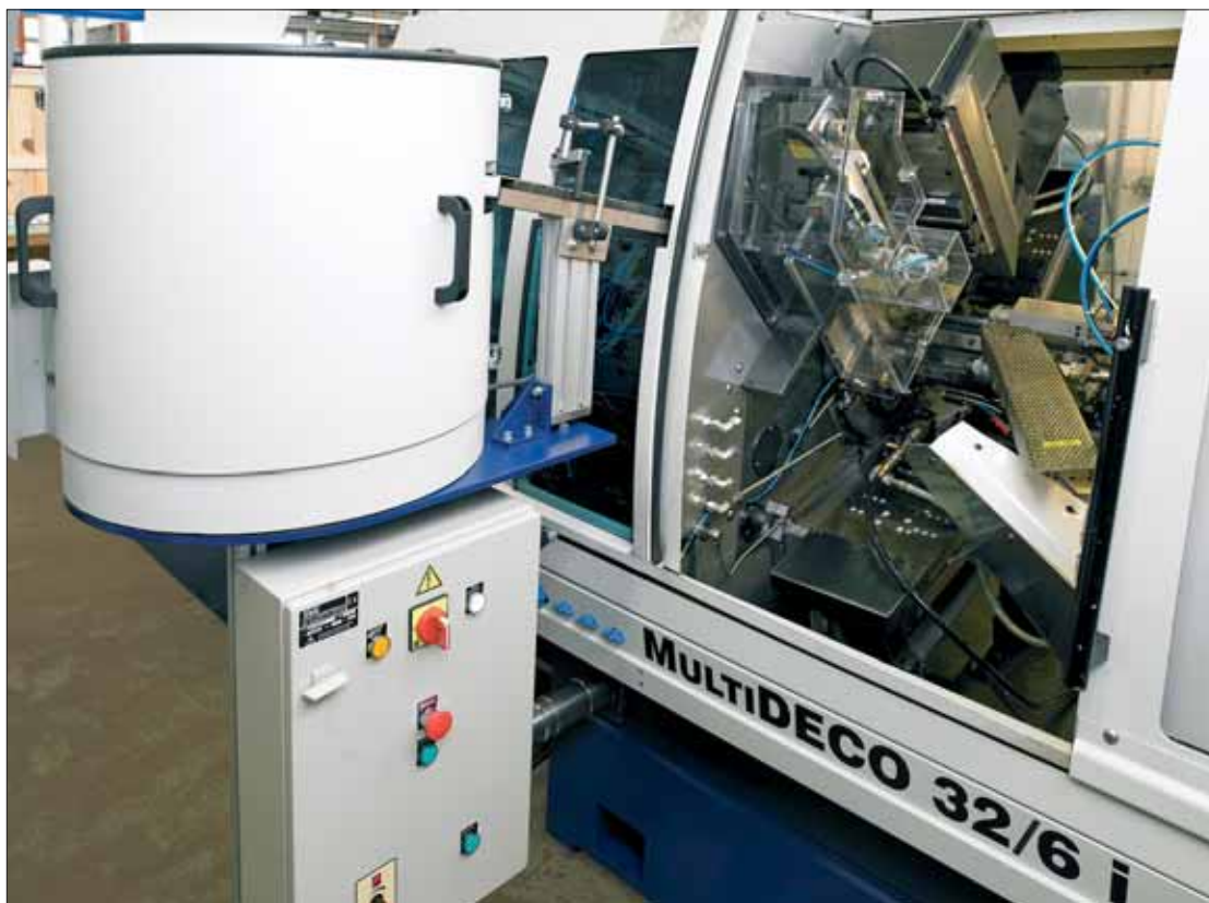
"Slide" feed system together with a vibrating bowl.
