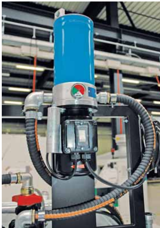
When pumping out used machining fluid, the fluid is cleaned to a particle size of 3 microns using an integrated and highly efficient pump. This means that optimum purity levels can be assured for the machining fluid in the used oil tank.
