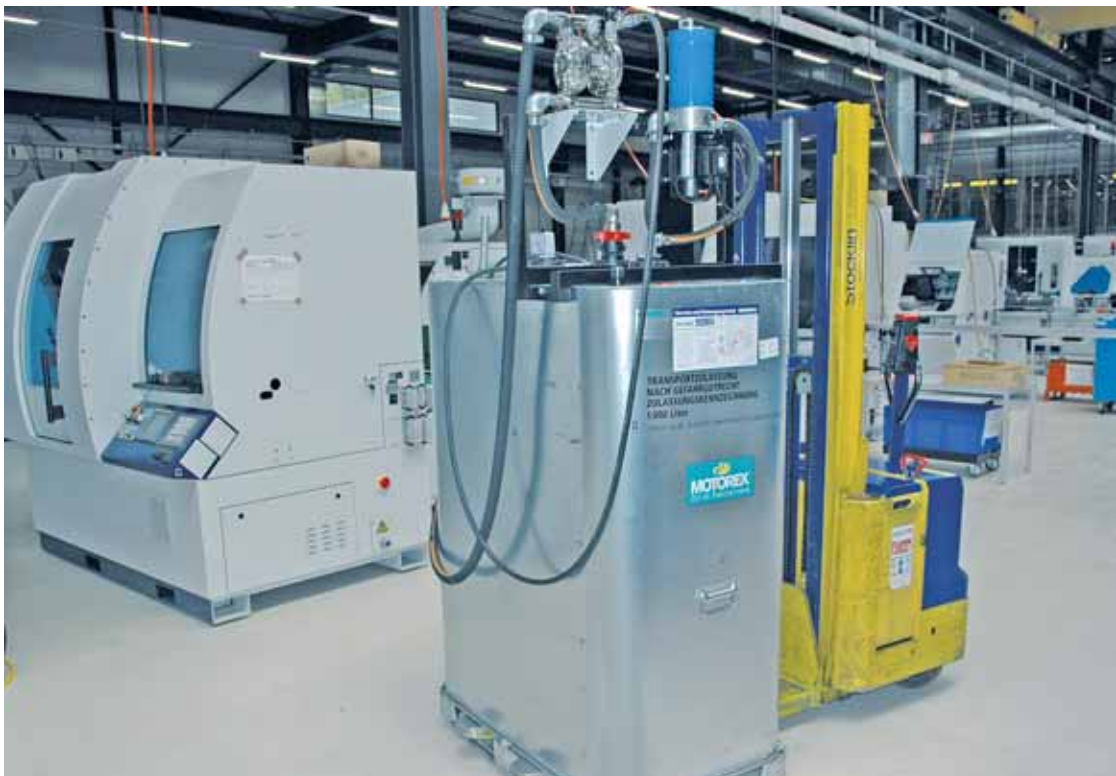
Several of these double-walled containers are available for filling and draining the machines. These can be transported like pallets and each one is equipped with a pump and a filter unit.
