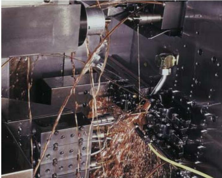
Parts are machined simultaneously on the top and bottom spindles of the DECO 2000 and many machining operations are performed at the same time also, virtually eliminating idle time and boosting productivity.
