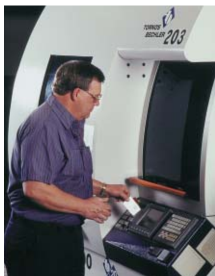
Tony Clark is about to download the program of the part, which is done on a desktop PC with the TB DECO software and stored on a magnetic card.
