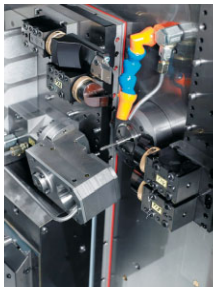
Machining area of the guide bush on the DECO 20a lathe with the external thread whirling unit, developed by TORNOS.
