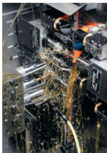
Productivity, performance, short setting up times on the DECO 20a due to 100 % pre-setting tool systems.
