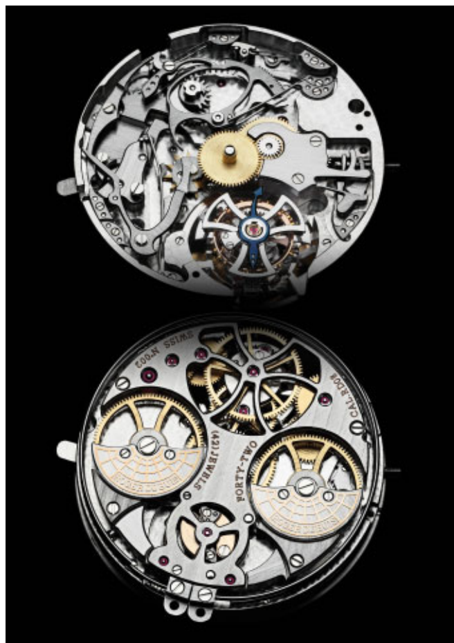
Round RD08 calibre, mechanical rewind with dual inertia-block, 14,000 lines, 42 rubies, rhodium-plated, "Côte de Genève" décor.
