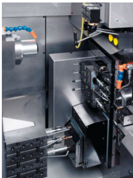
View of the machining area of the DECO 20a lathe fitted with the various pre-setting fast tool change systems.
