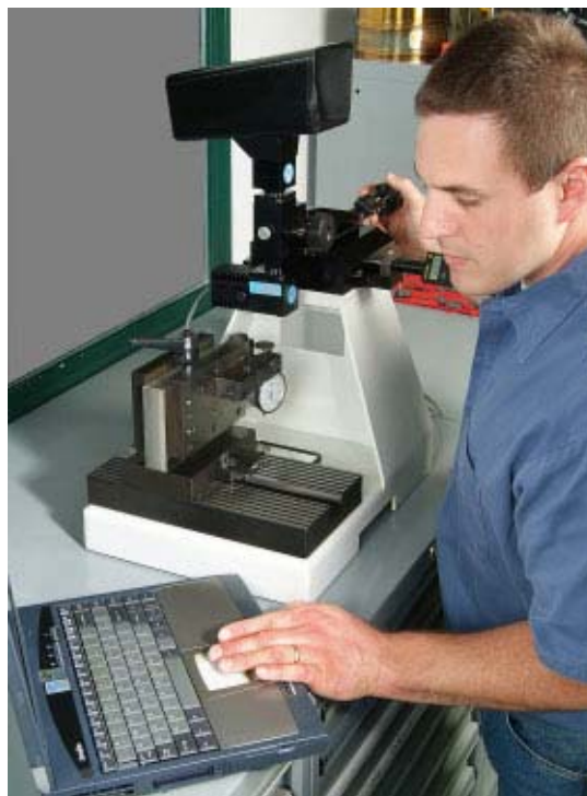
Tornos provides a tool presetting device with its DECOs to help set the tools for the next run while the machines stay in production.
