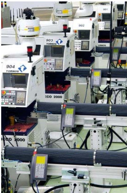
The company has eight Tornos DECO 10mm 9-axis machines to perform multiple intricate operations in a single setup. The ability to successfully perform polygon-milling operations on the machines is one of their hallmarks.
