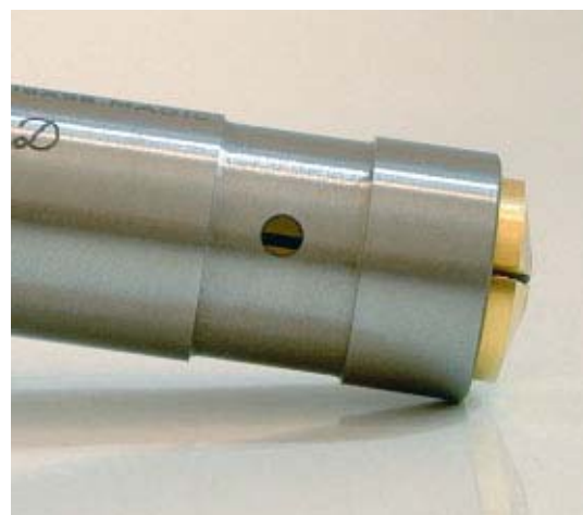
Additional oil ducts can be fitted to the side of most guide bushes on request. In this way, an adequate amount of lubricant can lubricate and cool the critical spots. Some suppliers provide their products with cross-holes as standard.
