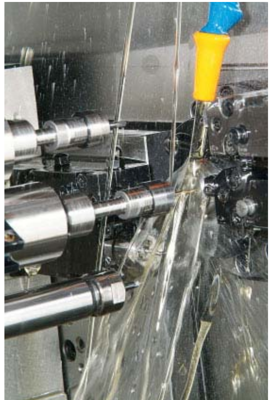
Interior view of one of the DECO machines; at top is the helpful polygon milling attachment.
