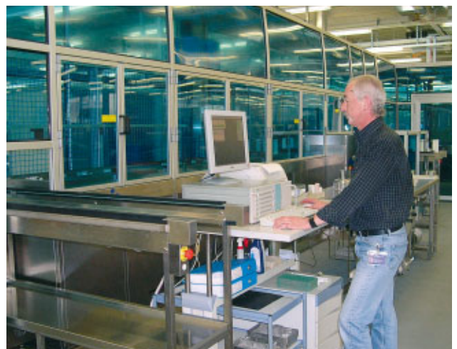
With various processes, the Amsonic AquaLine cleans complex components that are used for the medical sector and therefore need to be optimally biocompatible.
