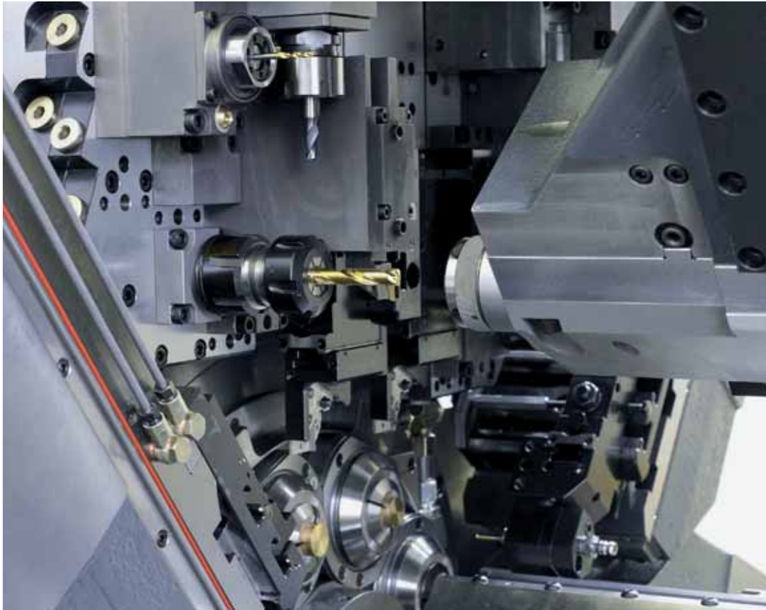
The two tailstock spindles, each mounted on separate axes, can be used to locate in the parts after the cutting-off operation and to machine their reverse sides (turning, boring, milling, etc.).
