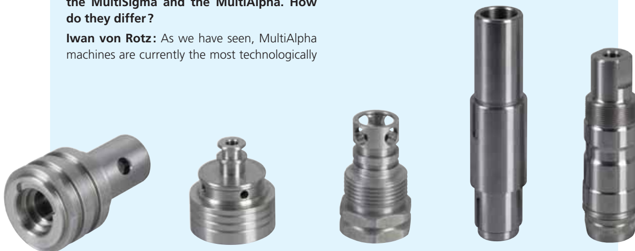
This type of part is now within the capability of a multispindle automatic lathe. It can even perform thread whirling operations!
