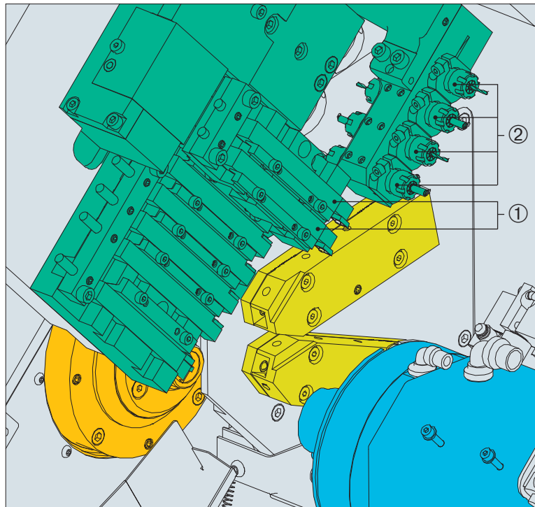
The positions for locating back-operation tools can also be used to accommodate a transverse drill. Pos. ① Cylinders with Applitec tool holders slide into their mountings to accommodate back operation drilling tools. Pos. ②
