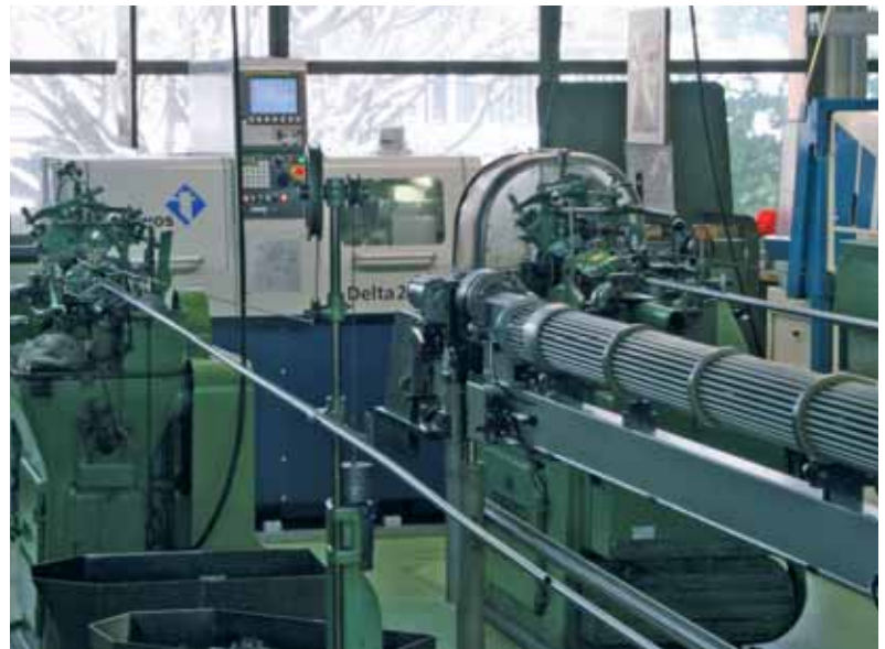
The Delta 20/5 is called up to gradually replace the cam-type turning machines.
