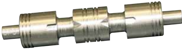
Typical MMT-machined workpiece. The number on the left side of the cylindrical section is engraved by the turning machine during machining operations.
