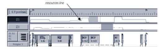
A speed value is displayed if you click on the red line. This value must be identical in both the small green flag – showing the start of the loop – and in the red flag – showing the end of the loop. Displaying the program as a GANTT diagram will allow you to determine when exactly a change in spindle speed or mode was programmed.
