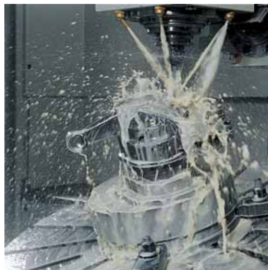
Cutting emulsions lubricate, cool and remove swarf – a substantial workload. (Photo: Blaser)
