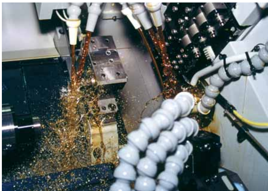
Cutting oils are an integral part of high-performance machining systems. (Photo: Blaser)
