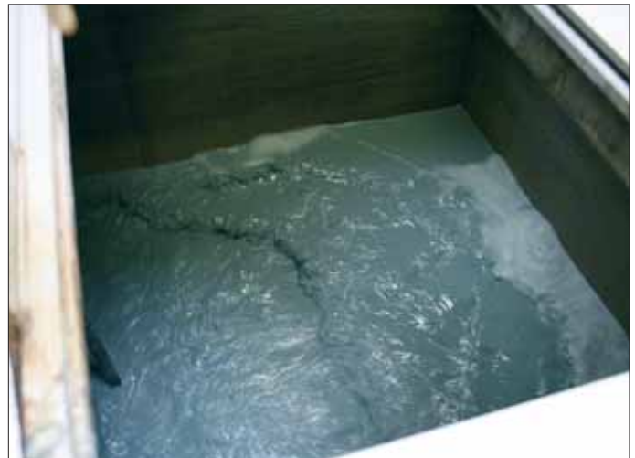
By mixing the used emulsions with a separating agent intensively, the emulsifier is less effective; water and oil separate more easily.
