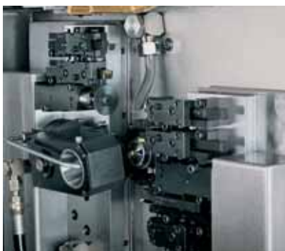
Thread whirling device on DECO 13a.
