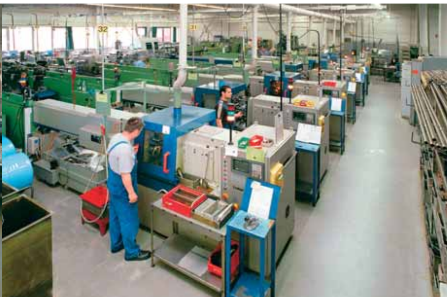
Standing in serried ranks: the Tornos CNC multi-spindle automatic turning machines and lathes in the Adelsheim plant.
