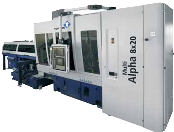
MultiAlpha 8x20: The first ever multispindle to use the thread whirling process.
