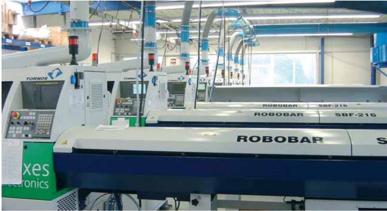
Standing in line are the eight Tornos CNC single spindle turning machines in Conec's modern production area.
