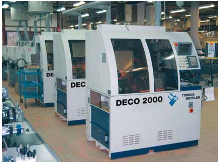
DECO workshop. In keeping with the multispindle units, each machine is linked to a centralised air purification system.
