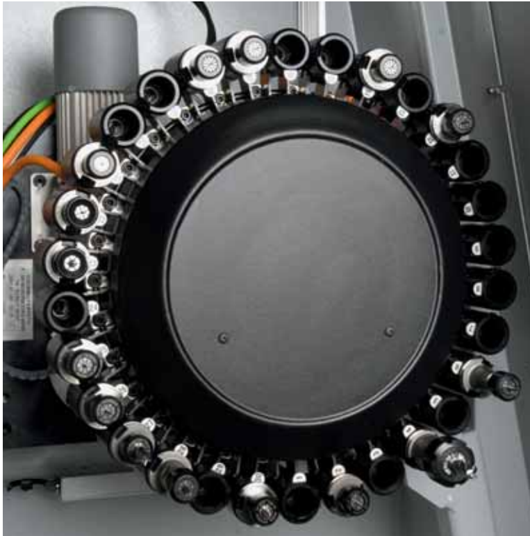
ISO 25 'Random' type 30-position tool changer
