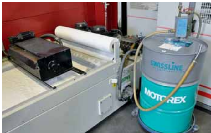
The leaked oil is skimmed off using the tape skimmer and the finest swarf and metal particles are filtered out by the tape filter. The compact, ever-necessary KSS mixing device is clearly visible on the mobile Motorex drum.
