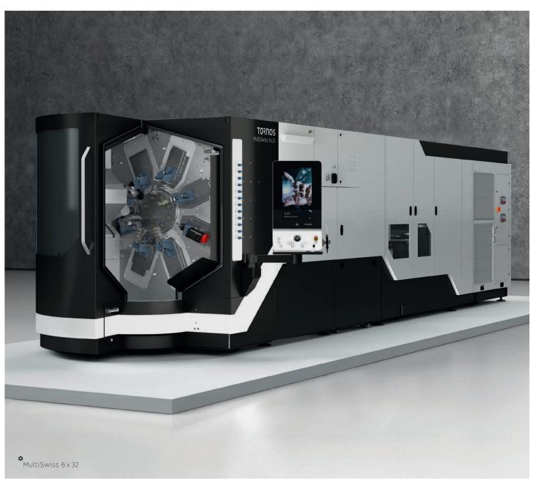
Cooling is integrated within the slides, which reduces the use of pipes which can not only be difficult to adjust, but also easily trap swarf. This concept makes the MultiSwiss as simple to set up as a single-spindle turning machine, the only difference ultimately lies in the number of collets to change.
