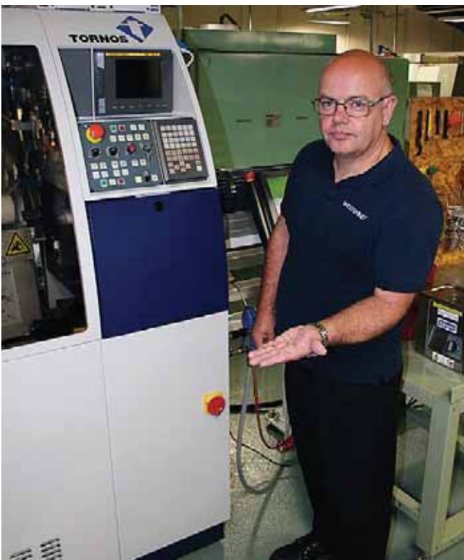
Steve Somers in front of Deco 10a holding some of the 2 mm long brass jets that are manufactured in quantities up to 30,000 per week.
