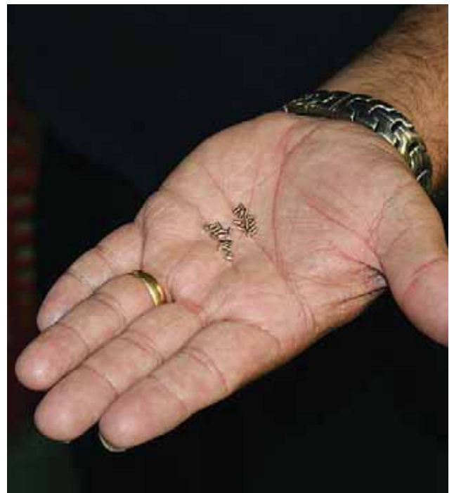
Close up of Steve Somers holding the 2 mm long brass jets that are installed into the high speed spindles
