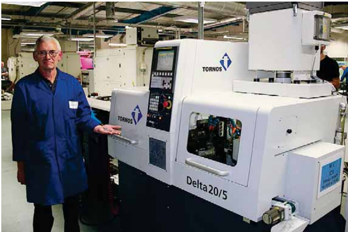
The Delta 20/5 and its operator holding screws, rivets, restrictors and development parts manufactured on the Delta.
