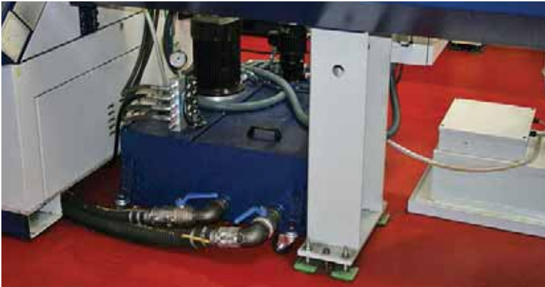
HPC pump retrofitted to Tornos Deco.
